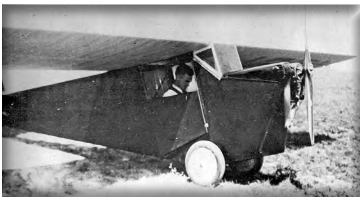
Eldon Cessna created the "Baby Cessna" by wrapping the CG-2 frame in a fuselage and a tiny enclosed cabin, adding wheels and a 25-hp Cleone engine.
