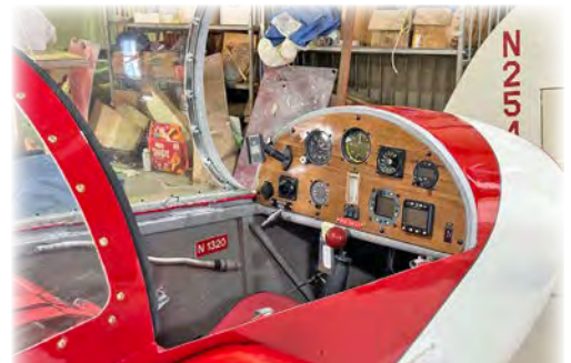
Instrument panel with Pfeiffer Pellet Vario.
