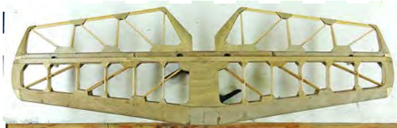
My chamfering and gluing of rib reinforcement leaves me with great admiration of vintage craftsmanship.
